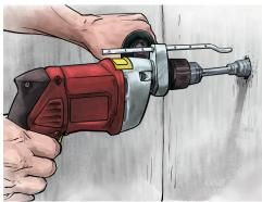
**3.** For larger holes, first trace the circumference of the desired hole. Then drill a series of holes around the perimeter of the tracing.
